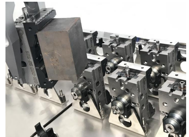
Indirect work piece handling by vises
